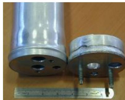
Fig 3.2: Comparison of MIG welding to MP-Weld in 6061-T6 Accumulator
