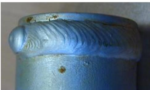
Fig 3.1: TIG Weld of Al6061 A/C R/D
