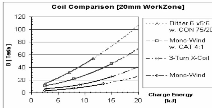
Fig 7.4: Distribution of magnetic field power in the axial direction as a function of coil type and bank energy
