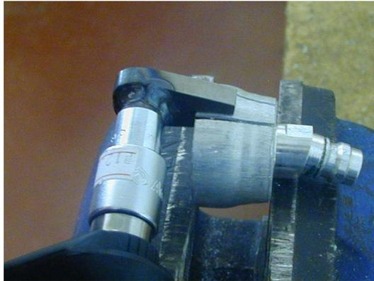
Fig 6.3: Torque tool head mounted for peel test
