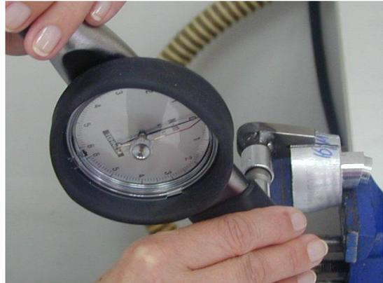
Fig 6.4: Torque tool being applied for peel test
