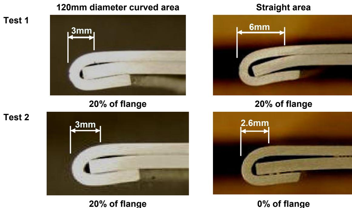
**Figure 8:** Deformation of the hem union for the straight area (left column) and the 120mm diameter curved area (right column) of the complex part for the First test (upper row) and the Second test (lower row).
