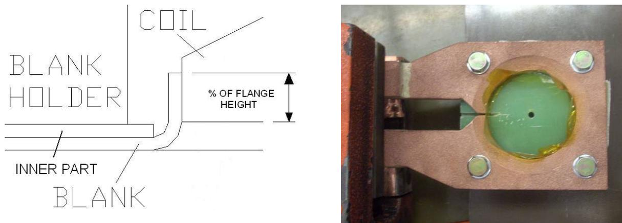
**Figure 3:** Partial section view of the circular hemming set-up with the % of flange height as input variable (left) and one of the hemming coils (right).
